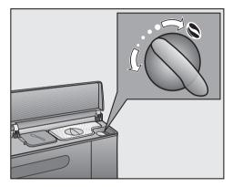
Turn the rotary selector for the grinder counter-clockwise for a finer grind or clockwise for a coarser grind.
